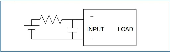
D. Recommended to use the circuit, the output peak voltage may cause SSR misoperation, so please add R/C circuit or varistor to absorb the peak voltage at the output end, see the following figure:
