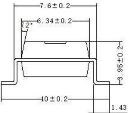
Note: No tolerance is marked as ±0.05mm.
